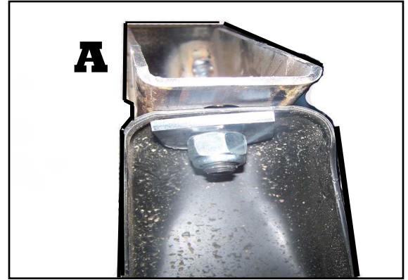
Side view of front level lok mounted on pad mount using reinforcing square washer.
